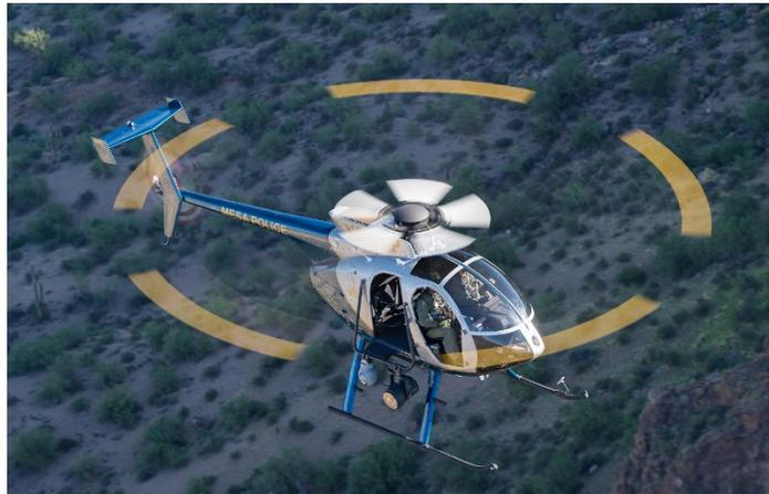
The MD 530F is certified for single pilot operations under visual flight rules (VFR)/visual meteorological conditions (VMC) and capable of training instrument flight rules (IFR) in VMC conditions. The MD 530F supports two crewmembers on the controls and two observers in the aft cabin. An integrated communication system allows all crewmembers and observers to communicate easily amongst themselves.
